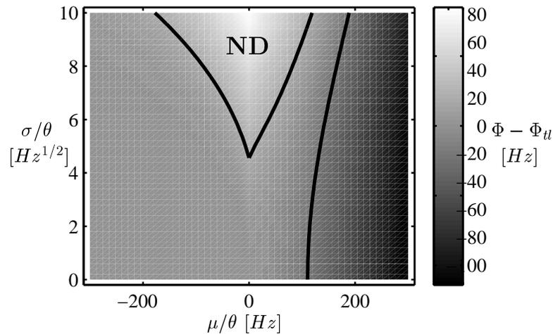
Figure 6: Difference between the aVLSI neuron current-to-rate transduction function  $\Phi(\mu, \sigma)$  and the threshold-linear function  $\Phi_{\ell}(\mu)$  in the space  $(\mu, \sigma)$ . Dark and bright regions correspond, respectively, to negative and positive differences (see the scale on the right). Contour lines are at differences of +20 Hz and -20 Hz. The two sources of nonlinearity are due to the absolute refractory period (for large  $\mu$ ) and the ND regime (the brightest region).
